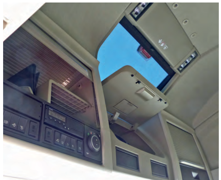
The front upper cabin features a large emergency exit and plenty of storage space behind blinds or flaps.
