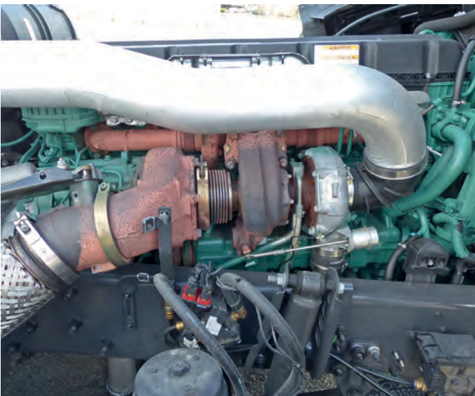
Two turbos are better than one, especially if the second one (left) acts directly on the crankshaft via a gear train and freewheeling. Volvo has perfected this turbo compound principle.
