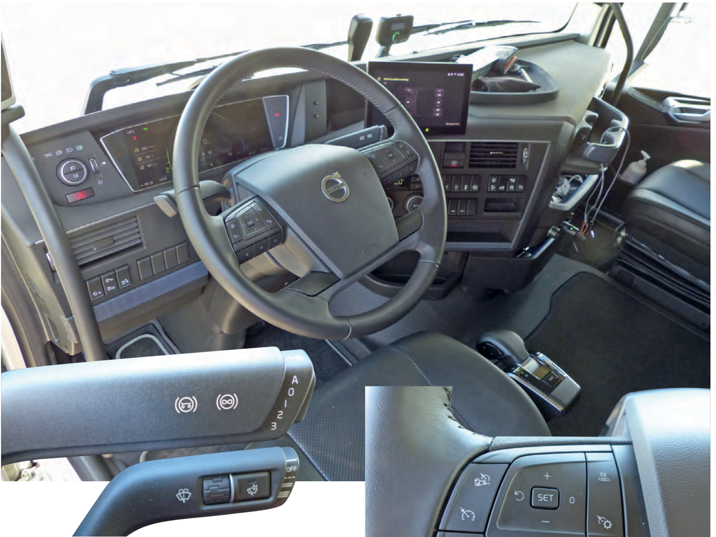
The engine brake and windscreen wiper levers are far too close together and still take some getting used to.
