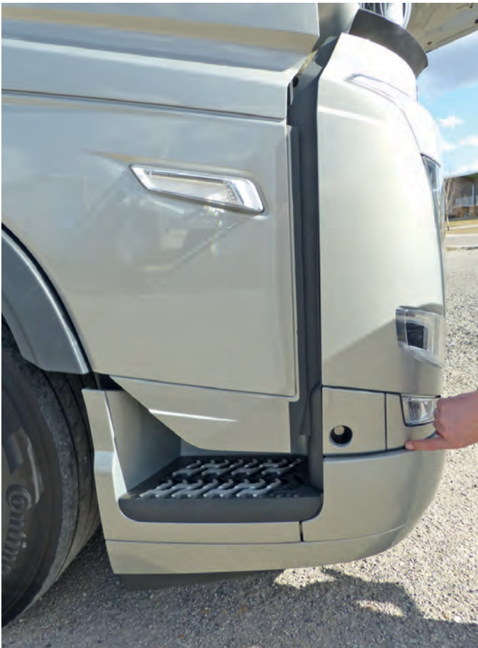
Tuning on all curves and roundings: Even smallest gaps are now sealed with gaskets. Especially the big gap which enables the cabins flexibility towards the fixed parts at the front.
