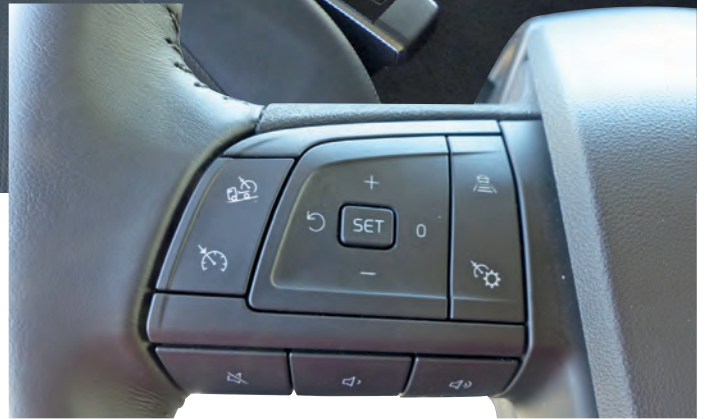
The steering wheel buttons on the left control all the cruise control functions, including the new downhill cruise control.
