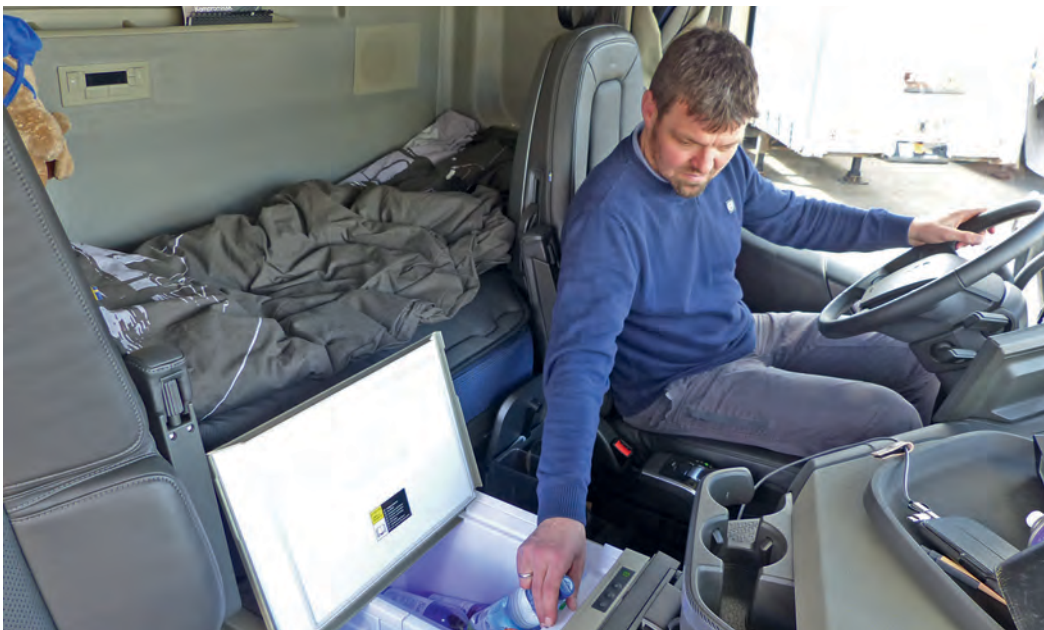
The FH's coffee maker is located between the driver's seat and the 33-litre cool box, but cool drinks are still within easy reach.
