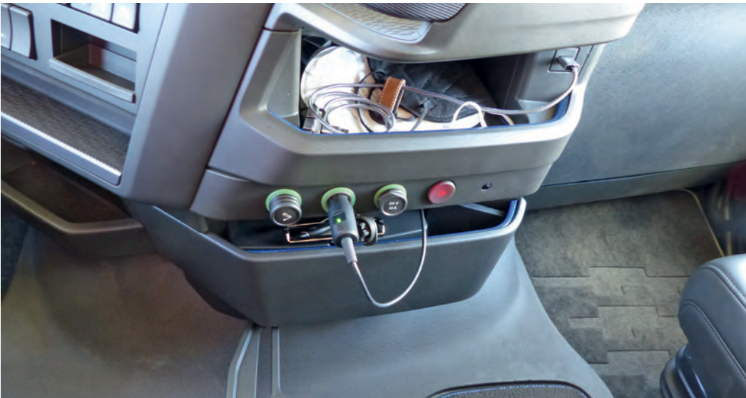
Three 12- and 24-V sockets are located in the middle, with a USB socket for a smartphone at the top. The red button activates the alarm system in the event of a robbery or an emergency.
