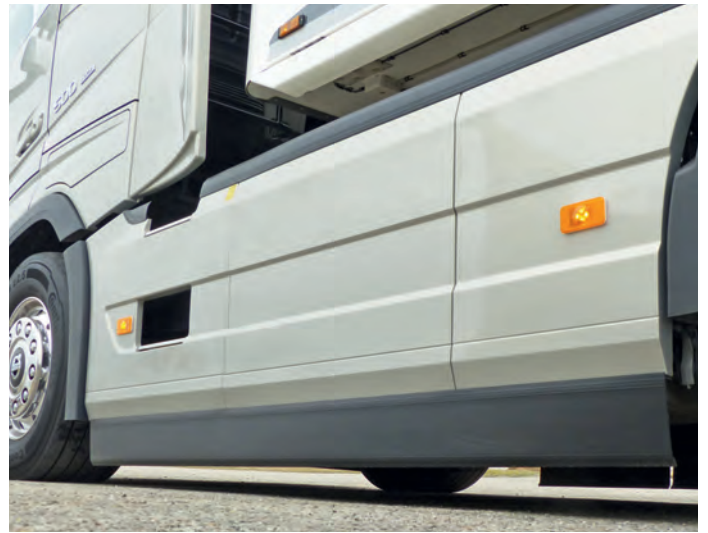
The enemy is air turbulence: New rubber lips on the side aprons leave only ten centimetres of clearance to the road, the mudguard mountings on the front axle narrow the gap to the tyres.
